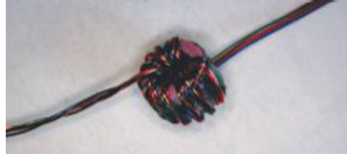
Shown here are the high-performance 10-GbE LAN transformer windings, which are made of twisted pairs.
